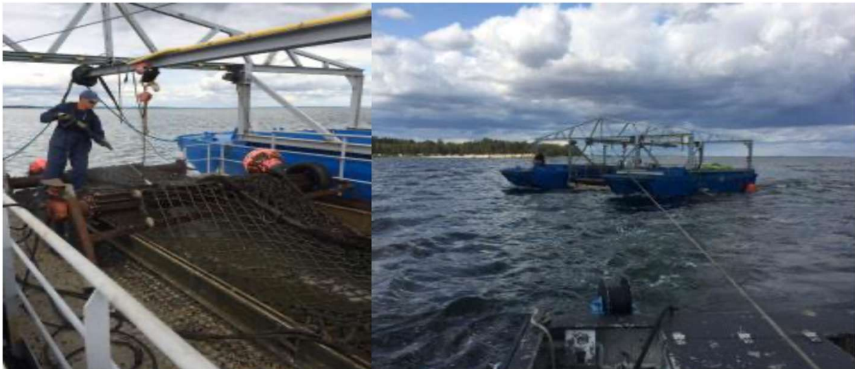
Figure 18: Harvest of a net farm (Hagby), using a catamaran platform to lift up the net and wash off mussels using a high pressure cleaner.
