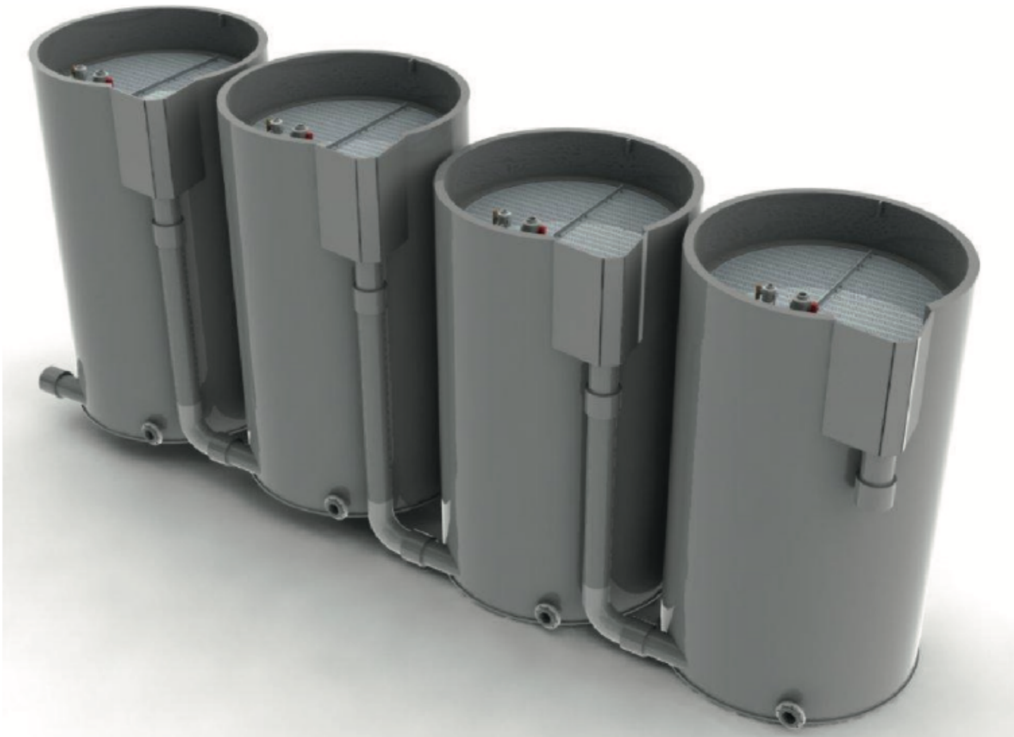
Figure 5.6 The flow pattern in the shown multi chamber PE biofilter goes from left to right and upstream in each chamber. Most of the organic material is removed by heterotrophic bacteria in the first chamber. The consequent low organic load in the latter chambers secures a thin nitrifying biofilm for converting ammonia to nitrate. The last chamber is called a microparticle filter and is designed for removal of very fine particles that have not been removed by the mechanical filter. Source: AKVA group.
