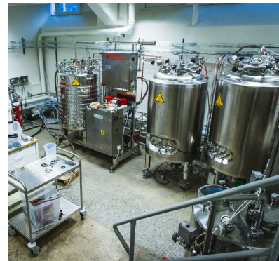
Pilot bioreactors (50 and 600 L)
