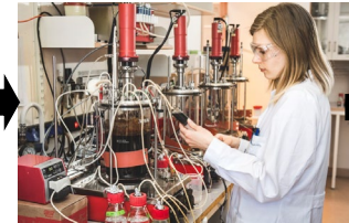
Lab bioreactors (4x3 L)
